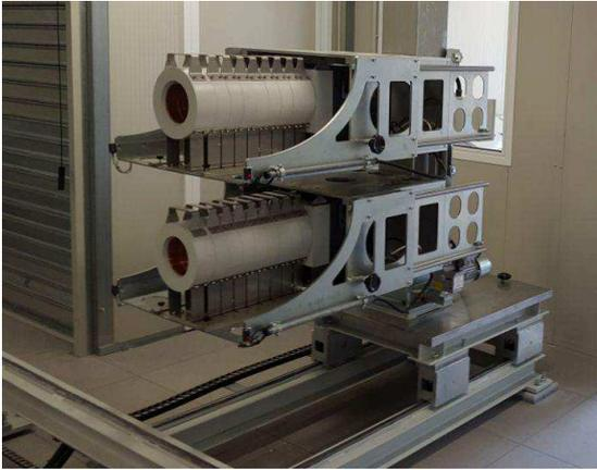
The movement sequence takes place through a computer-controlled automatic procedure, which places the platform into three different positions: loading area, weighting/measurement area and unloading area. Two tower detector assemblies are positioned on both sides of the container and the detector-to-container distance can be adjusted manually.
