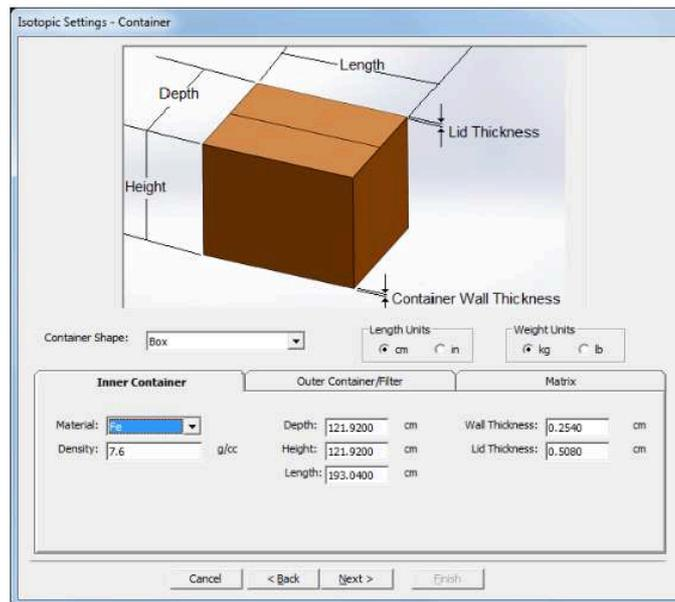
Container configuration for detector positioning.
