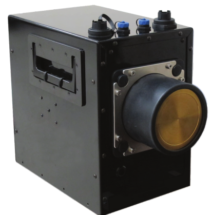
AURAS electro-cooled HPGe example
