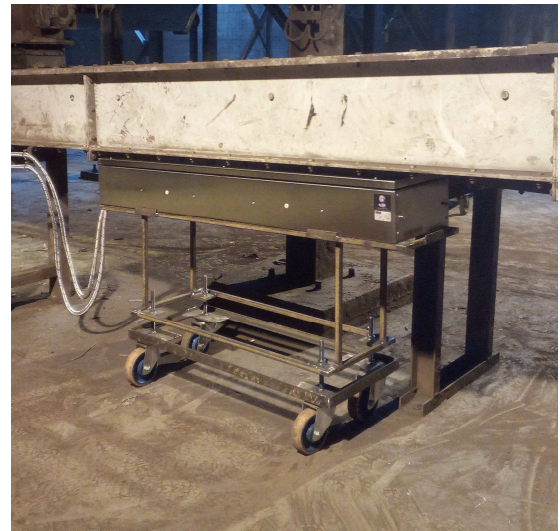
Specific application: monitoring of materials carried on conveyor belt
