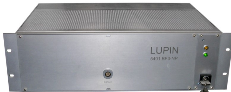
Optional: radiation sensitive electronics installed in a separate rack
