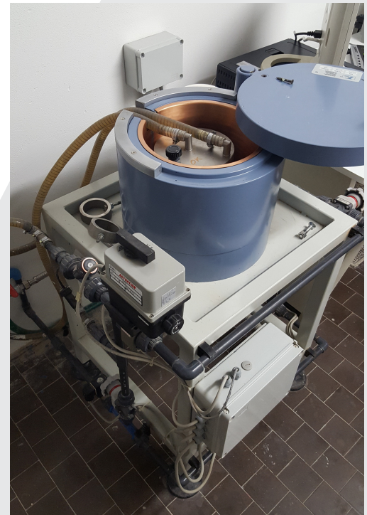
Marinelli geometry measurement chamber inside lead well
