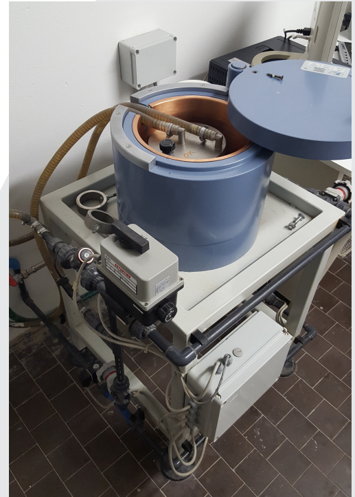
Marinelli geometry measurement chamber inside lead well
