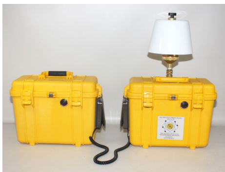
Air Sampler Connected to a Portable Battery Bank
