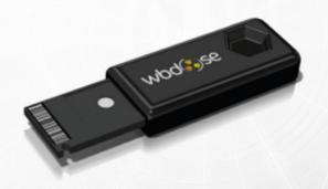
Each dosimeter includes IDs codified by RADKOR. It is easier to register wbdose dosimeters and tracking them. wbdose dosimeter's size is quite suitable for whole body dosimeter usage. Wbdose dosimeters consist of BeO crystals (Zeff=7.11). Those dosimeters, which have OSL characteristic, are delivered to users as calibrated and ready for use.
